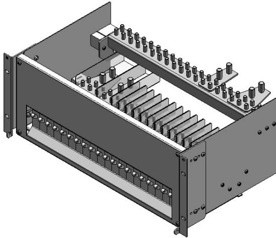
The DCM2000 DC distribution provides circuit protection for a wide selection of telecommunications loads up to 250A per circuit and 800A per distribution. All circuit breakers are alarmed through auxiliary contacts providing voltage-free alarm signals. The DCM2000 is designed to comply with recognized international standards and for complete operator safety. Full front access is provided to allow easy termination of load cables in either vertical or horizontal cable entry.
